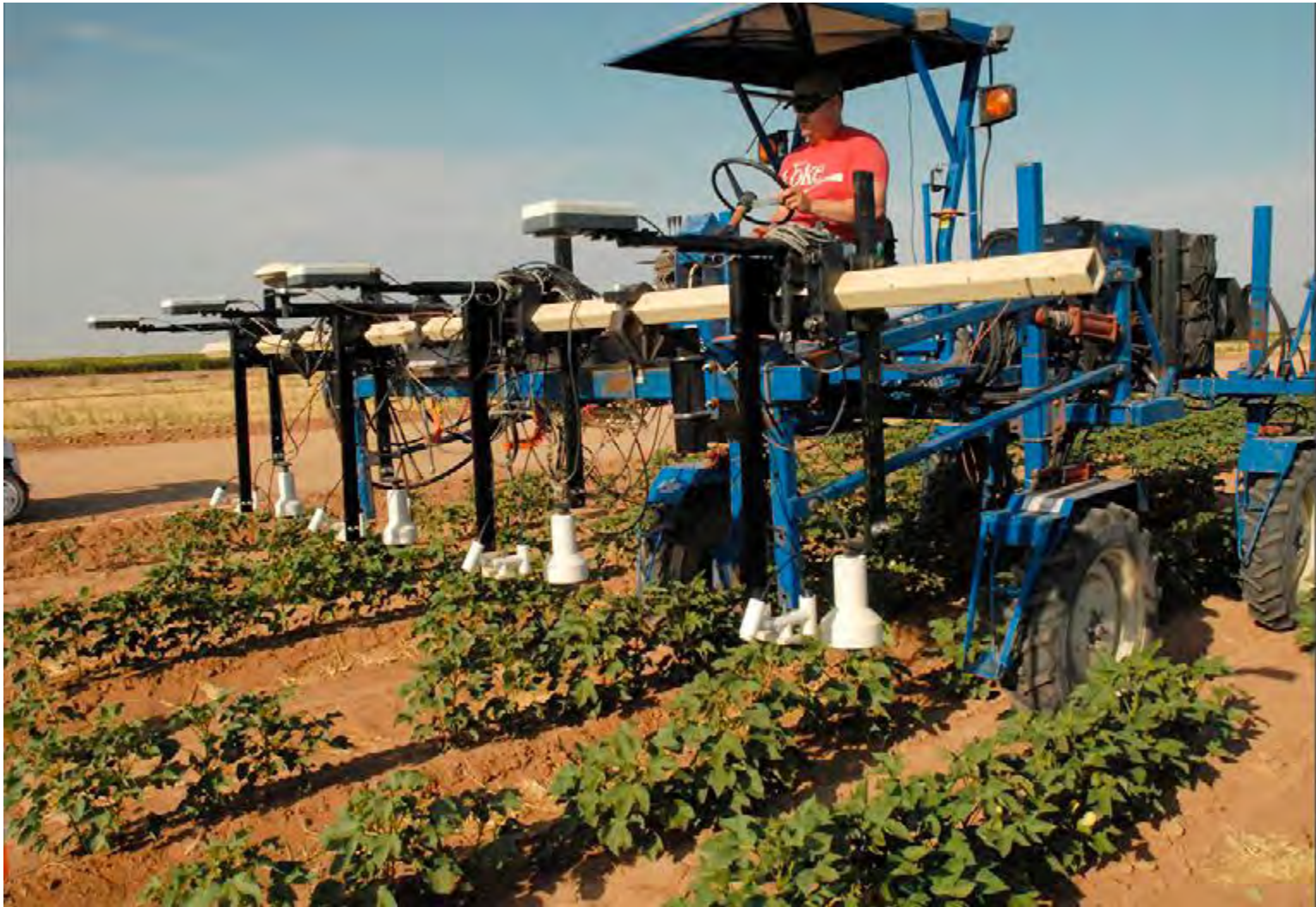
Fig. 1. High-clearance tractor in operation over young cotton plants at Maricopa, AZ. Replicated sets of sensors allow simultaneous measurement of canopy height, temperature, and spectral reflectance at three bandwidths. Real time kinematic GPS provides positional accuracy under 2 cm.
