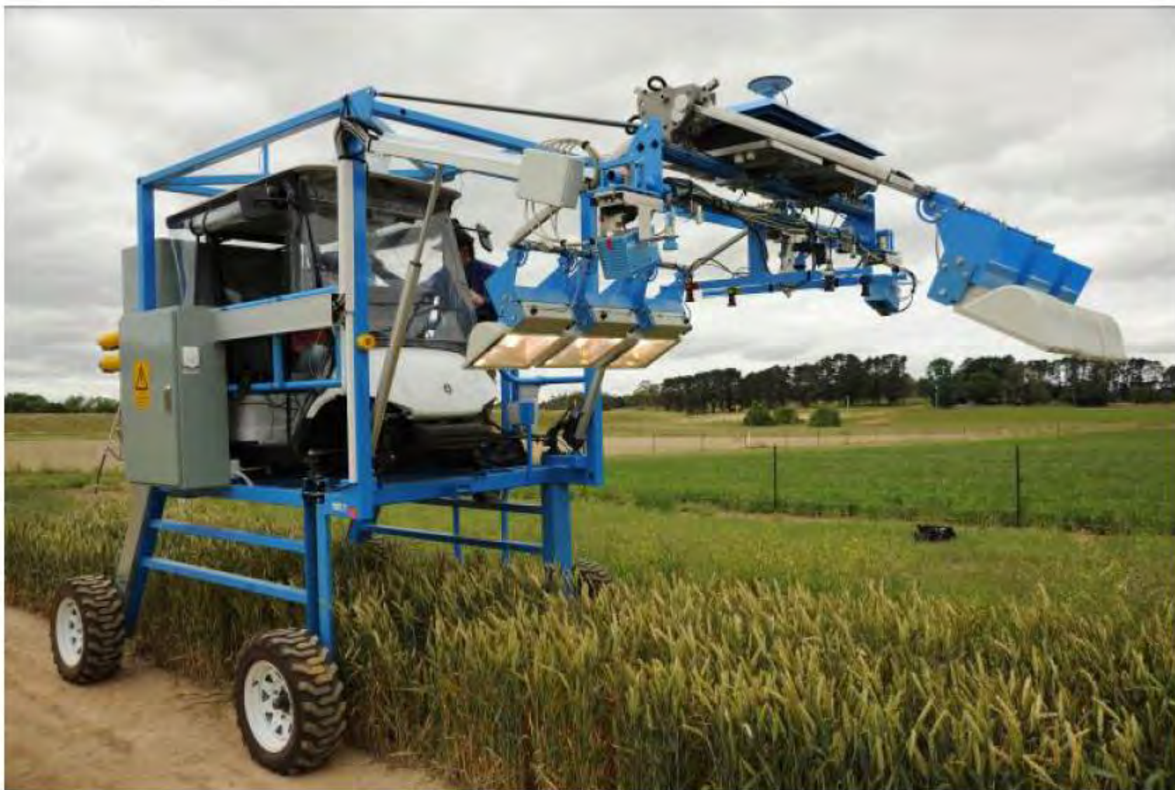
Fig. S3. Purpose built crop monitoring buggy fitted with: four RGB cameras for measurement of ground cover and plant establishment; LiDAR sensors to measure plant height and bio-volume; spectral radiometer from 300 to 2500 nm to measure NDVI and various spectral vegetation indices; three infra-red temperature sensors for crop canopy temperature. Rebetzke et al. 2013 FPB 40: 1-13
