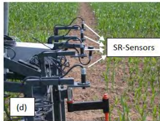
Fig. S1. (a) Front and (b) back view of the sensor platform in driving position and closer view of the (c) light curtains (LC) and (d) spectral reflectance (SR) sensors.
